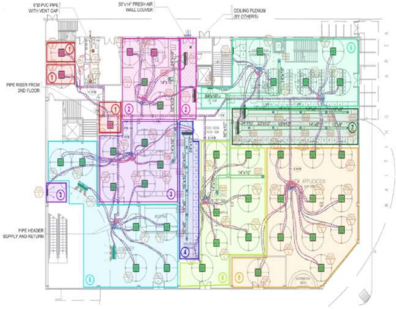
GRD FLOOR AC LAYOUT PLAN SCALE 1:500 METERS BIM SCALE REFERENCE 0m 1m 2m 3m 4m 5m
